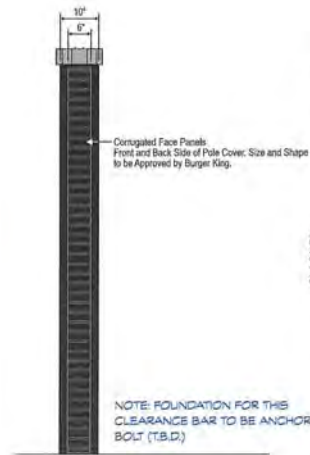
Front View - S-10.1A Clearance Bar Scale 1/2" = 1'-0"
